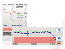
**Trend software** feature including configurable alarms alerting users of changes to the nerve response during continuous vagus monitoring
